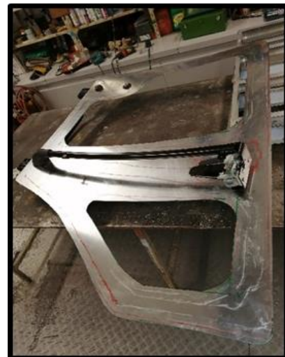
Marking for latch and handle on the door frame
