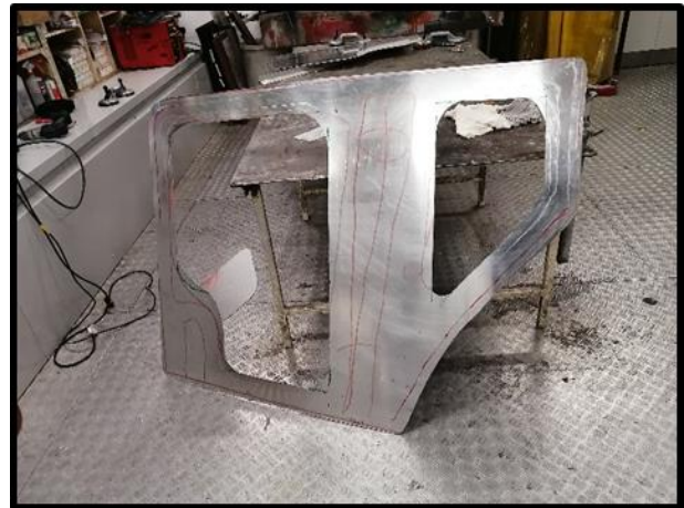
Fabrication of door frame in process
