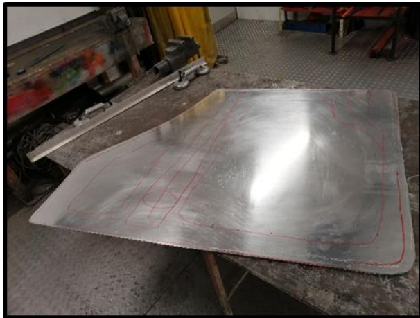
Markings on the sheet metal for cutting
